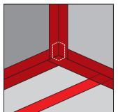
When corners are to be protected with a RESISTO MEMBRANE, gussets (a small piece of membrane) must be installed first to waterproof the corners.
