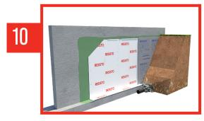
It is recommended to install a protective panel, such as SOPRA-XPS, if the soil contains clay, or to protect the membrane during backfilling.
