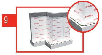
Finish by adding a bead of elastomeric sealant to the top and bottom of the membrane.
